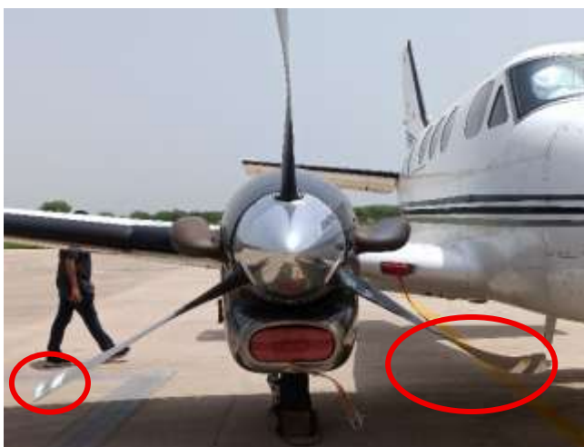
FIG 2: Damage to RH Propeller
