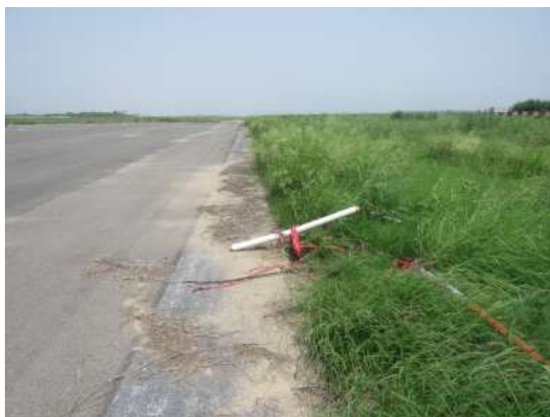
FIG 9: Location of Far Field Monitoring Antenna after the incident
