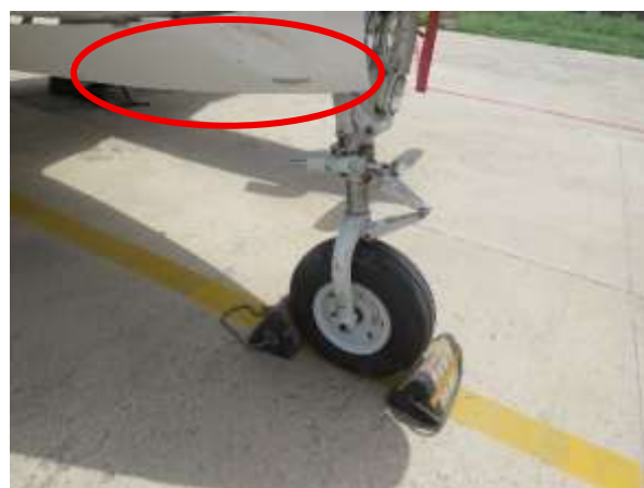
FIG 4: Damage to Nose L/G
